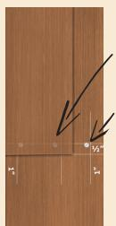
Use 2 fasteners for 4", 5", and 6" wide shingles
